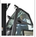
A partial cabin offers optional windshield with wiper, roof with reading light and rear panel with wiper. Soft doors can be added. A hard cabin option features clear view doors, 2-way sliding windows and heater option.
