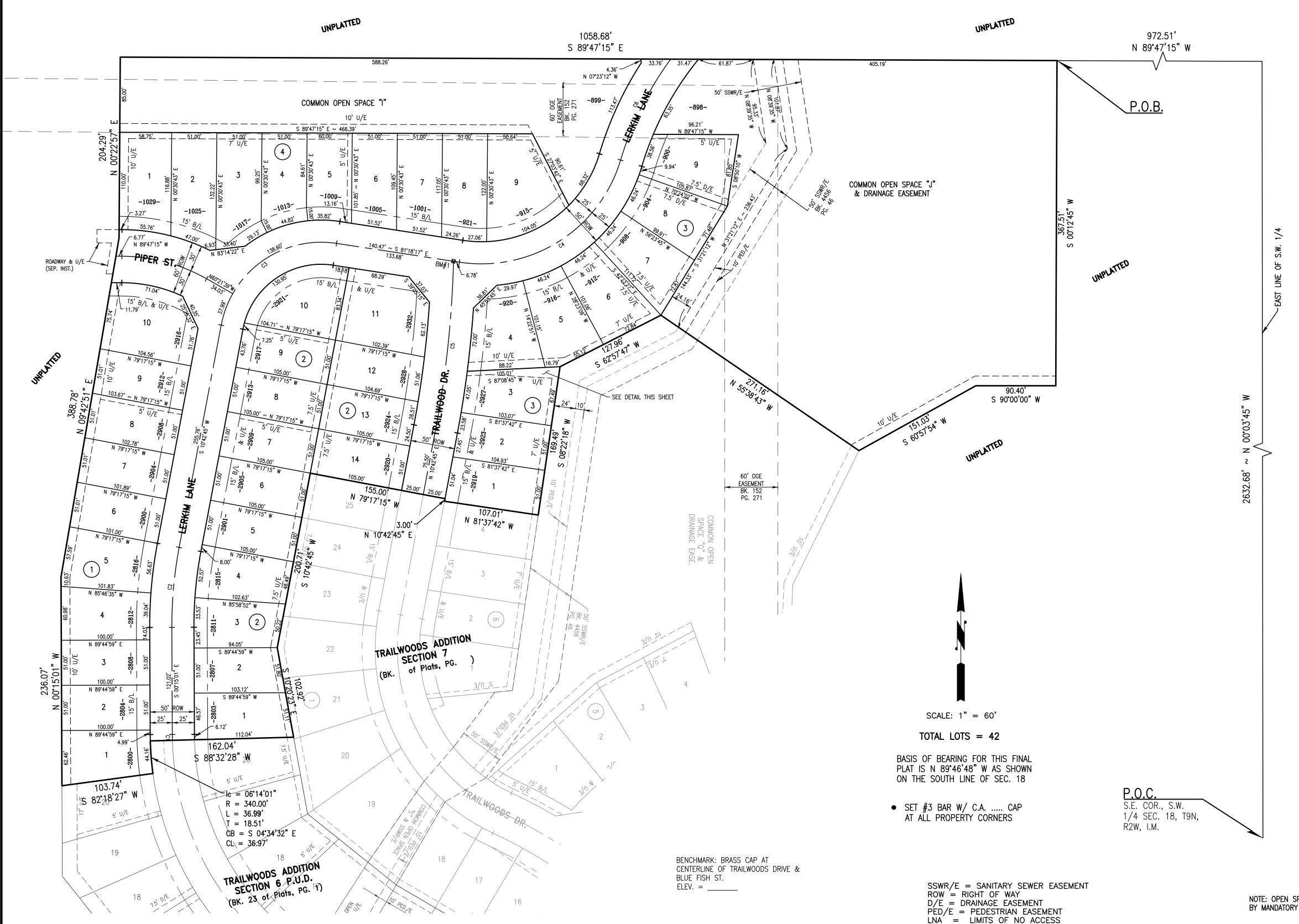
NOTE: THE UNIT OF MEASUREMENT SHOWN FOR ALL DIMENSIONS ON THE FINAL PLAT IS U.S. SURVEY FEET.
