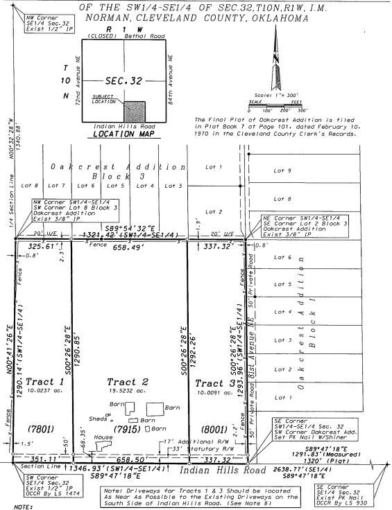
Bearings Shown are Based on an Arbitrary Bearing of S89°47′18″E Between Existing Monuments at the Southwest and the Southeast Corners of the SE1/4 of Section 32, T10N, R1W, [.M.
