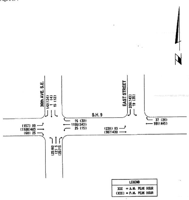
The model was used to determine the length of lane storage required for the eastbound projected left turning traffic at both the 36<sup>th</sup> Avenue SE and the Bellatona Boulevard intersections and is shown in the following figure (Figure 1) provided by TEC as part of TIA. The schematic also shows the 1,285 feet separation between the 36<sup>th</sup> Avenue SE and Bellatona Boulevard intersections.
