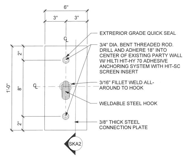
\*NOTE: CONTRACTOR SHALL PROVIDE EXTERIOR GRADE QUICK SEAL PRODUCT DATA TO STRUCTURAL ENGINEER FOR APPROVAL.
