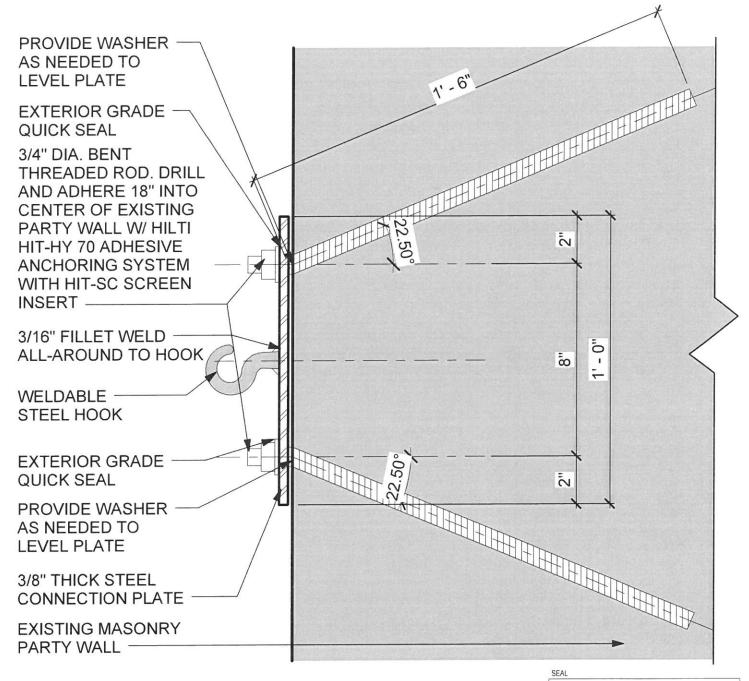
\*NOTE: CONTRACTOR SHALL PROVIDE EXTERIOR GRADE QUICK SEAL PRODUCT DATA TO STRUCTURAL ENGINEER FOR APPROVAL.
