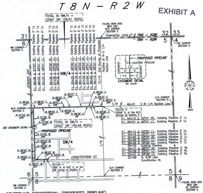
CENTERLINE DESCRIPTION: (PROPOSED PIPELINE) BEGINNING at a point 669 feet North and 542 feet East of the Southwest Corner of Section 5, T8N - R2W,
