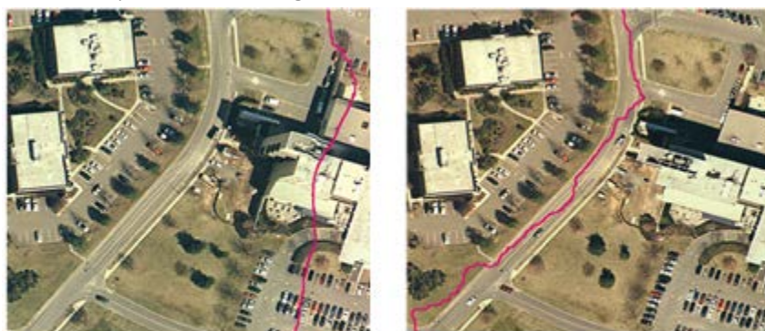
Orthophoto mosaic without intelligent seams (left) and with intelligent seams (right).
