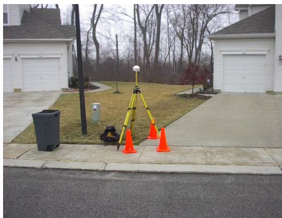
Example of a photo ID control point (intersection of driveway with sidewalk) that could be utilized.
