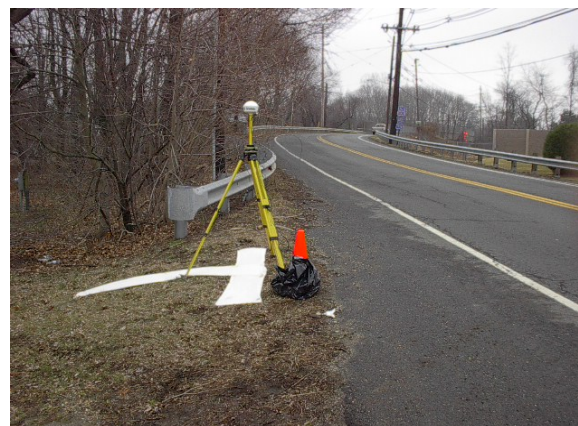
Example of a targeted control point
