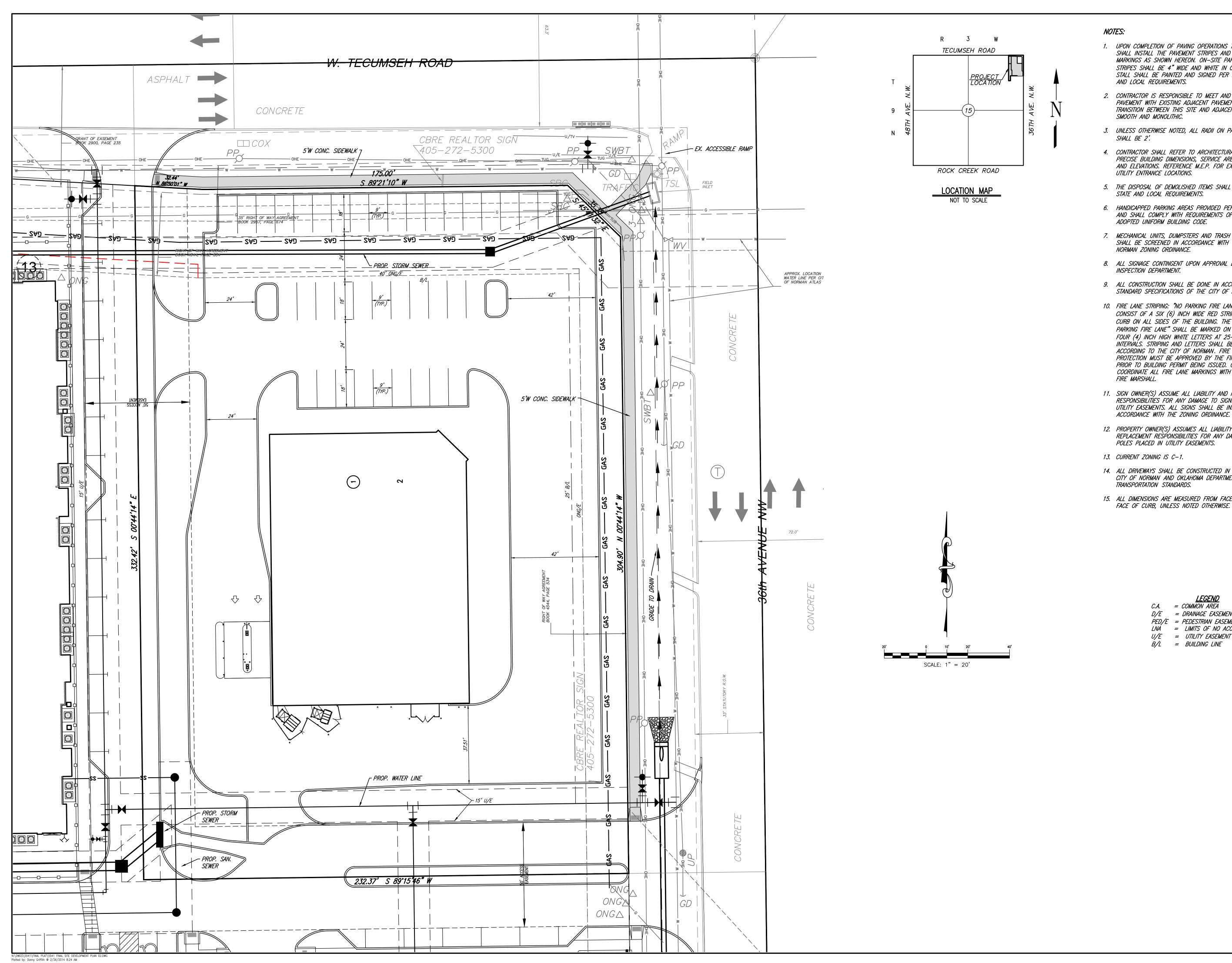
1. UPON COMPLETION OF PAVING OPERATIONS THE CONTRACTOR SHALL INSTALL THE PAVEMENT STRIPES AND PAVEMENT MARKINGS AS SHOWN HEREON. ON-SITE PARKING STALL STRIPES SHALL BE 4" WIDE AND WHITE IN COLOR. HANDICAP STALL SHALL BE PAINTED AND SIGNED PER FEDERAL, STATE, AND LOCAL REQUIREMENTS.
