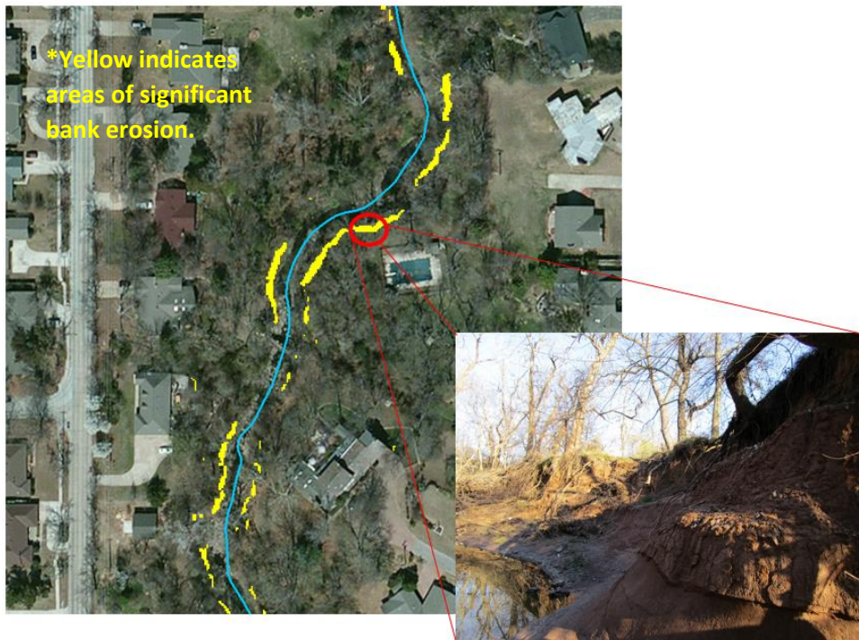
Figure 3: Example of Site Problem Area
