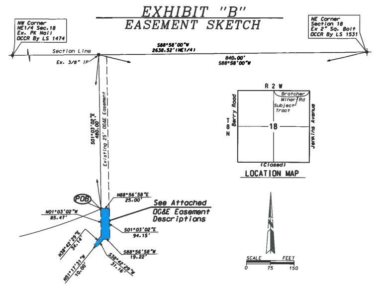
Note: Bearings Are Based On S88\*58'00"W Between Existing Monuments at the Northeast and Northwest Corner of the NE1/4 of Section 18. T8N. R2W. I.M. ( • ) - Indicates Existing 1" Iron Pin Or Monument as Noted. ( OCCR ) - Indicates Oklahoma Certified Corner Record On File Or To Be Filed With the Oklahoma Department of Libraries. Archives Division.
